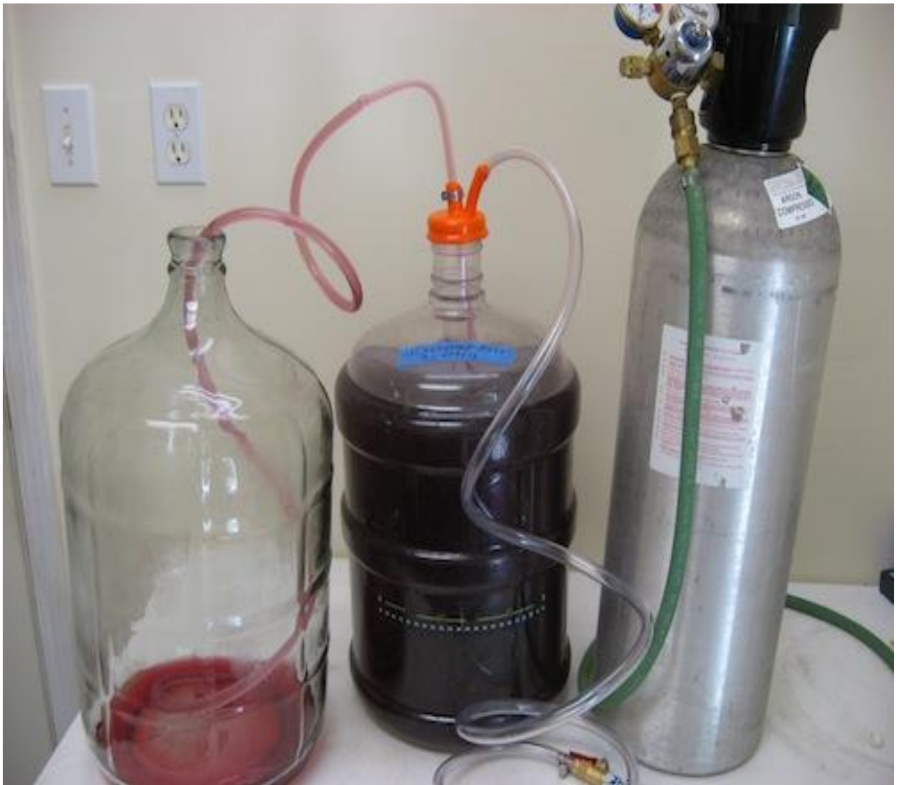
Figure 12: Inert gas system
